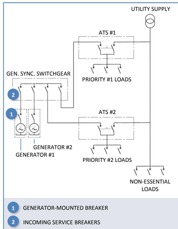
*Figure 1. A multiple-generator power system with industry-standard fault protection and prioritized loads*
